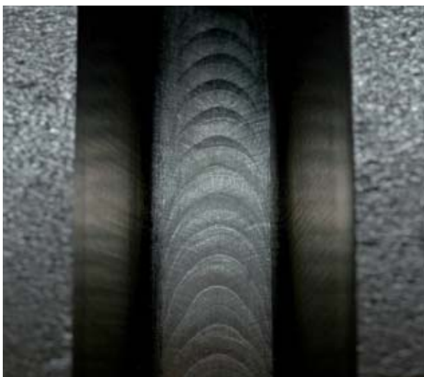
Figure 1 16-8-2 Outside view of weld root on TP 316 Cb
